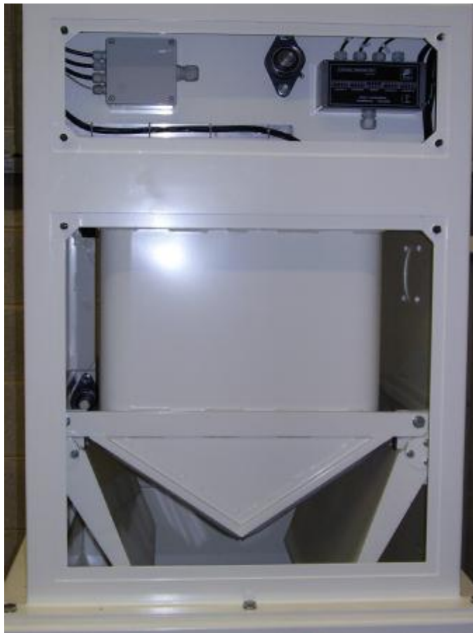
Figure 5 Location of the load cell junction box
