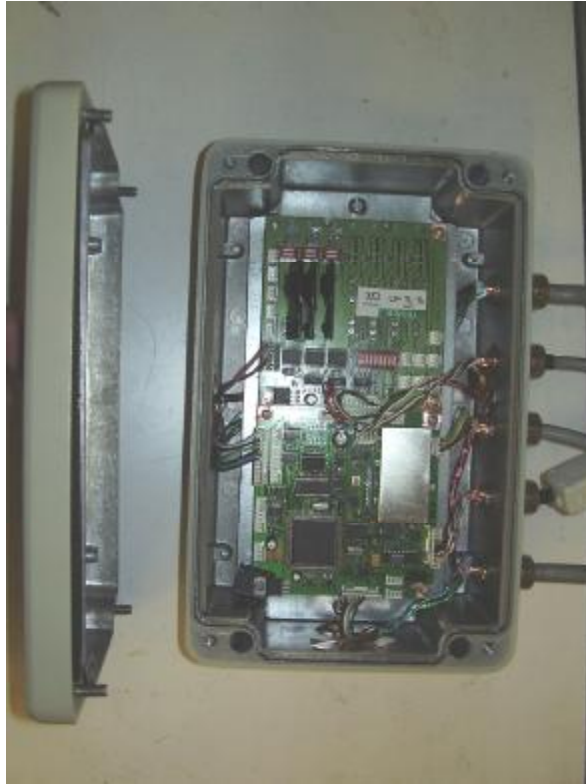
Figure 4 Control and I/O boards in enclosure
