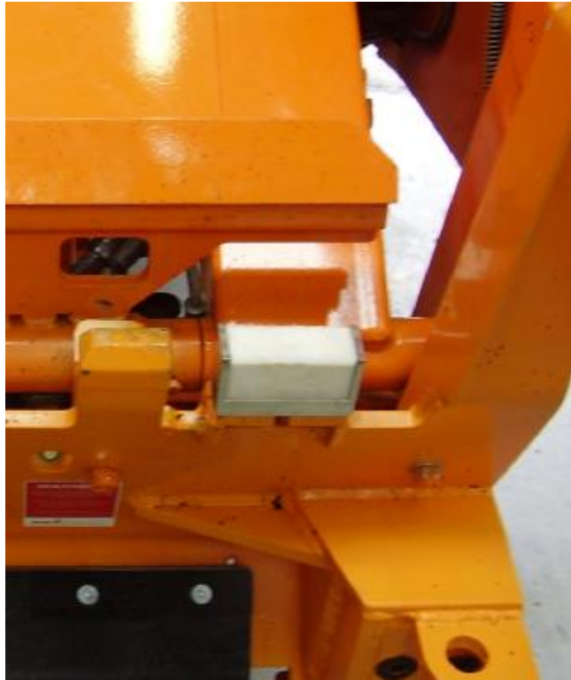
Figure 6 RFID antenna at rear of vehicle
