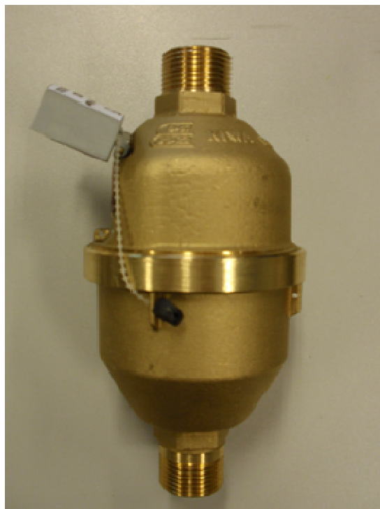
Figure 22 Sealing of V100 Larger Lid with Laser etched markings
