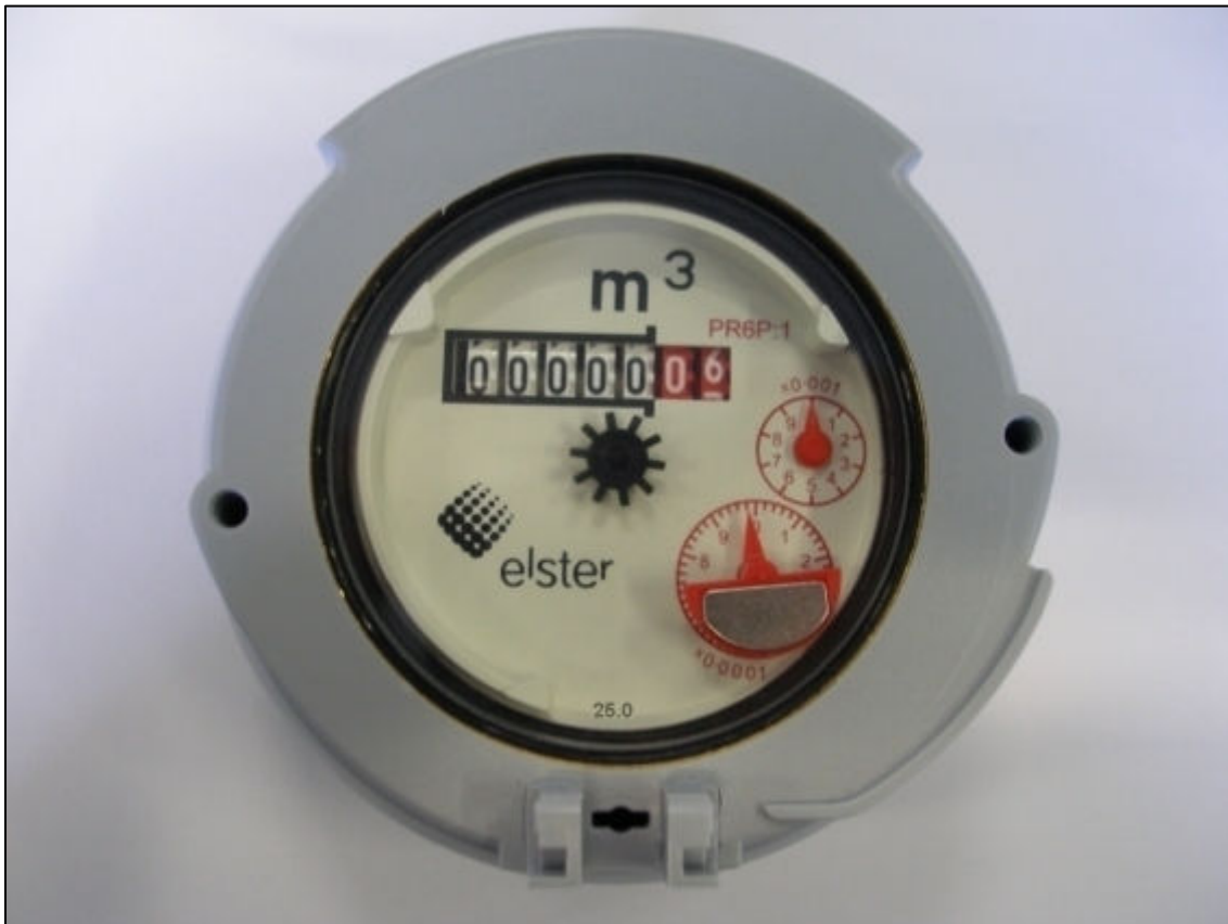
Figure 15 Standard register with additional copper can spacer clamp ring
