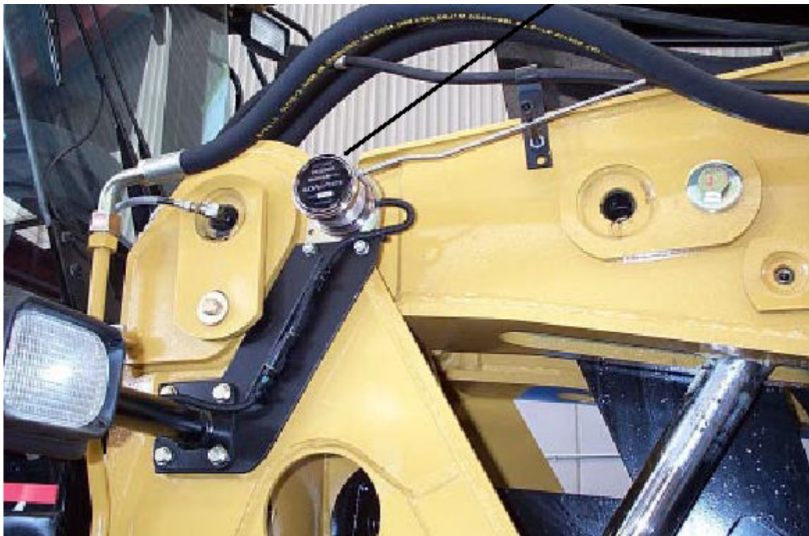
Figure 4 Typical LR908 sensor installation
