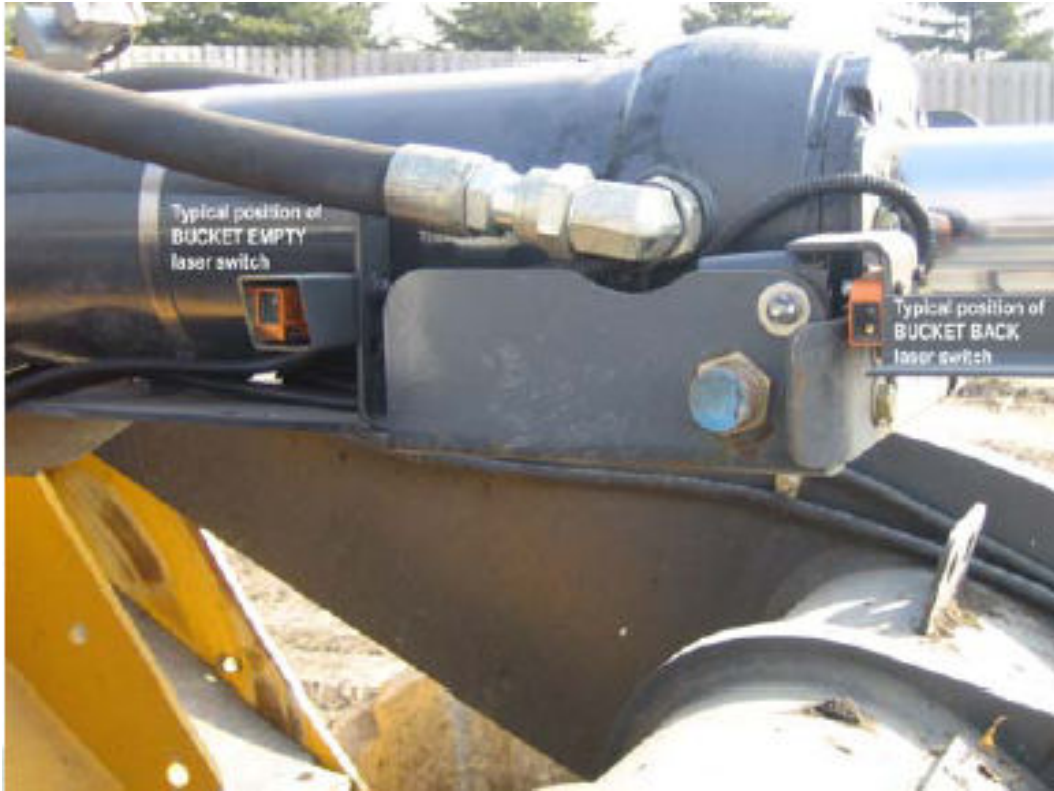
Figure 5 Typical AAA-20710 “crowded back/forward” location sensors
