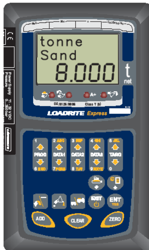
Figure 10 Loadrite Express LR917 Legal for Trade System indicator console
