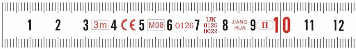
Figure 5 Example of the pattern with markings
