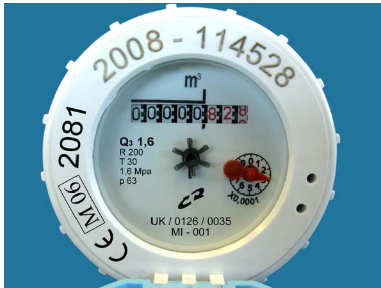
Figure 5 Top Face of meter showing verification markings
