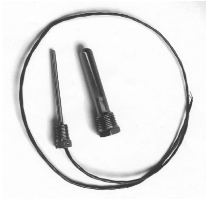
Figure 7 Temp Probe and Sealing arrangement
